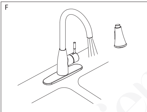
F. Turn on water supply to check for leaks at all connection. Remove spray head from the pull out hose and let the water run for about 1 minute and check for leaks. Reattach the spray head.
