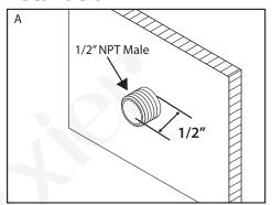
A. Shut off the main water supply before installation. The faucet requires an 1/2" NPT threaded male nipple extending 1/2" from the finished wall. For ease of future maintenance, it is recommended to install a shut off valve for the water supply line at an easily accessible location.
